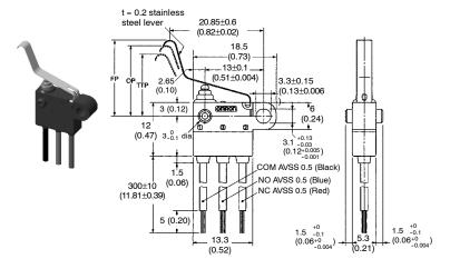
**Note:** Dimensions not indicated in the above diagrams have a tolerance of  $\pm 0.2$  mm.
